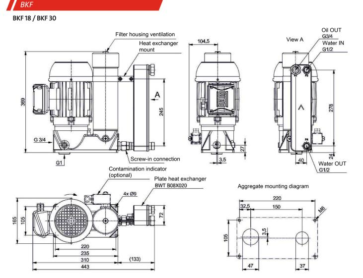
**Note:** When installing next to the oil reservoir please not the intake! When determining the bores on the reservoir be sure the contamination indicators remains visible!
