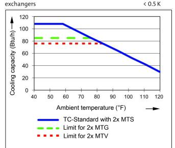
Note: The limit curves for the heat exchangers exchanger PTG, PTV or MTV apply to a dew point of 104 °F.
