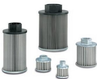
Installed upstream of the pump, or in the intake line with a contamination indicator accessible from the outside for particularly easy maintenance, our suction filters ensure that the pump is highly safe from coarse contaminants. A wide selection of elements suitable for every system protect installations and pumps in the fine range of 10–25 µm with our mic qualities, or in the coarse range with cleanable wire fabric.
