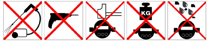
Fig. 4: Prohibited mechanical stress
