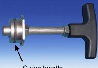
Attach an O-ring suitable for the expected ambient temperature to the handle. Attach the downstream filter to the handle. Then carefully insert the handle with filter in the gas probe and turn 90° to secure. Verify the handle is seated correctly. When seated correctly it locks onto the filter housing.
