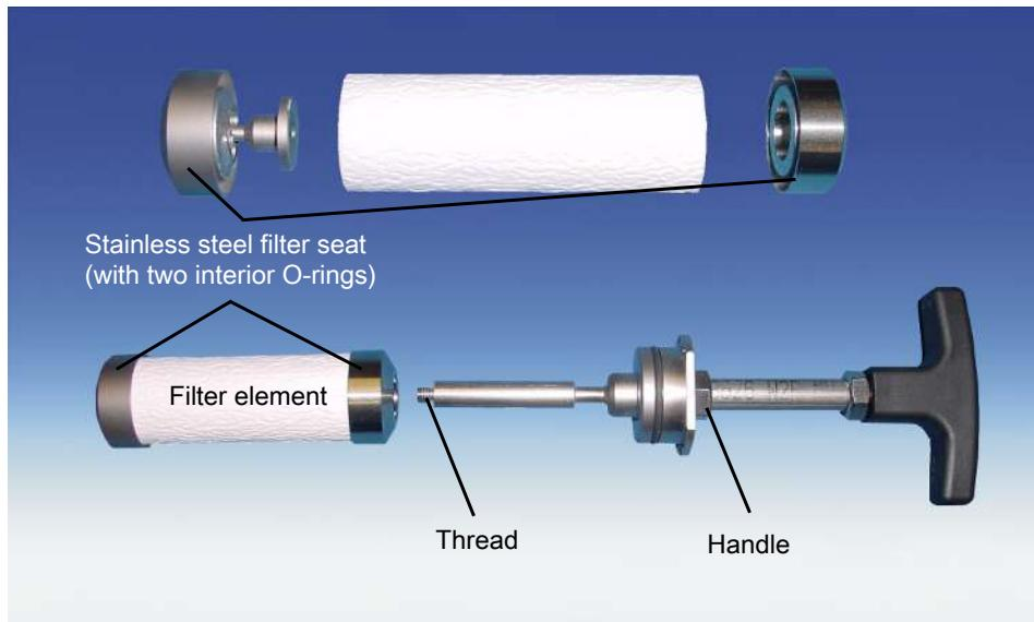
With the filter removed, you may also clean the inside of the sampling tube if necessary by blowing it out or using a cleaning wand.
